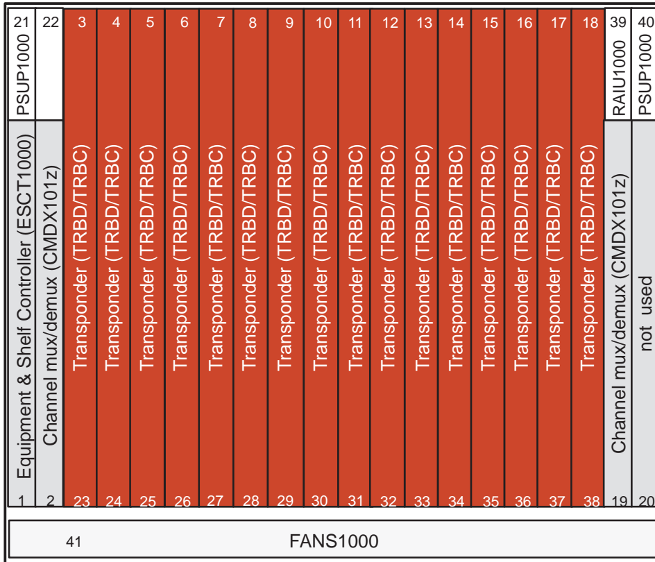
Figure 41. Example of a slave/transponder shelf configuration
